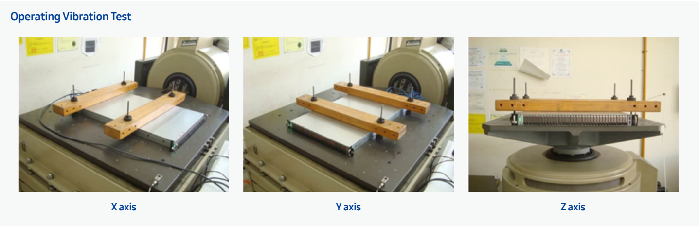
Figure 25: Vibration Testing Setup
